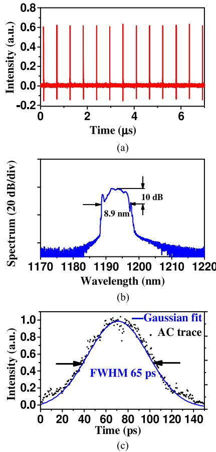
Fig. 3. (a) Pulse train, (b) output spectrum, and (c) autocorrelation trace of the mode-locked laser at a pump power of 900 mW.
