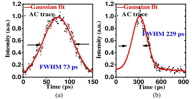
Fig. 6. AC trace of the mode-locked laser with total cavity length of (a) 160 m and (b) 200 m.
