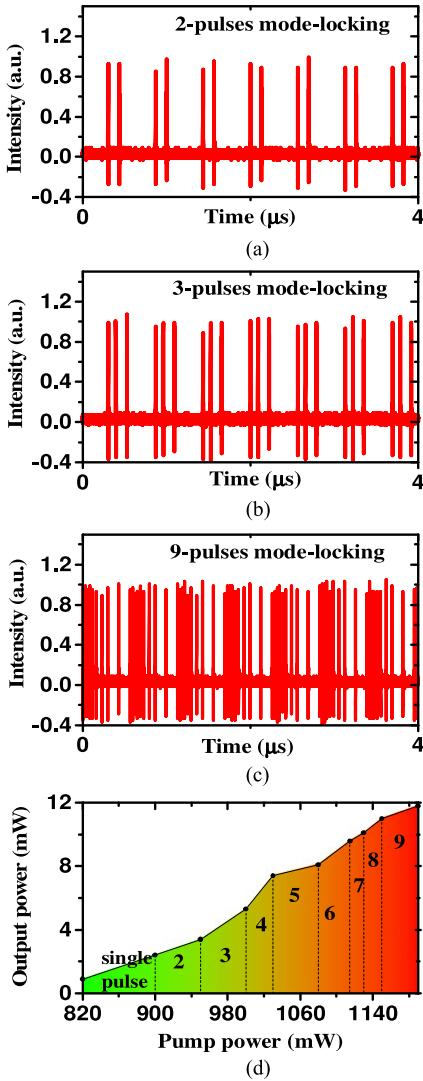
Fig. 5. Typical pulse trains of mode locking states with 2(a), 3(b), and 9(c) pulses. (d) Output power and states of the mode locking as a function of pump power.
