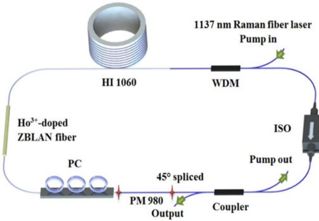
Fig. 1. Experimental configuration of the mode-locked Ho<sup>3+</sup>-doped ZBLAN fiber laser.
