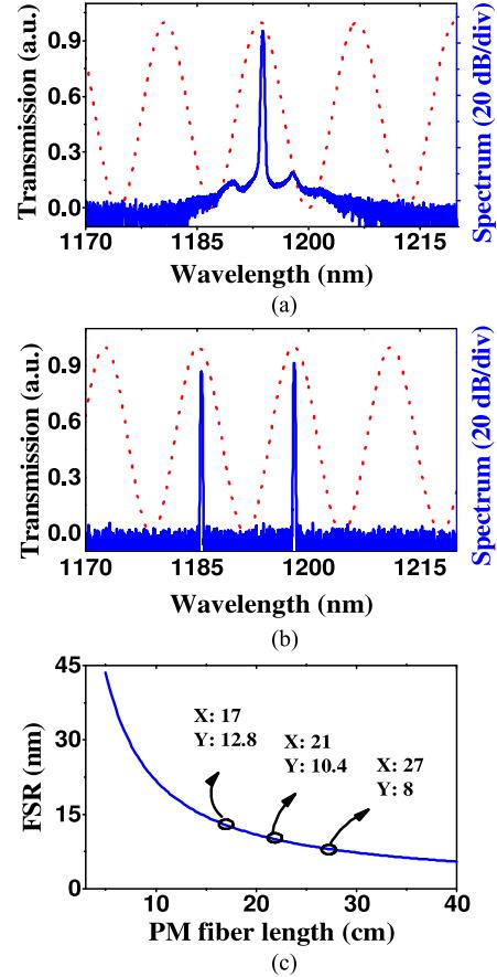
Fig. 2. (a) Single wavelength operation of the fiber ring laser. (b) Typical optical spectrum (solid blue curve) of dual wavelength operation of the fiber ring laser and the simulated transmission of the Lyot filter (dotted red curve). (c) Measured FSR of the Lyot filter for 17, 21, and 27 cm PM fibers and the calculated FSR of the Lyot filter as a function of PM fiber length.
