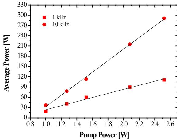
Fig. 2. Average output power versus launched pump at different repetition rates.
