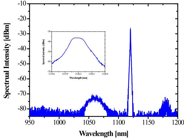
Fig. 5. Spectral characteristic of the 1120 nm Q-switched fiber laser. Inset, detailed spectrum at 1120 nm.
