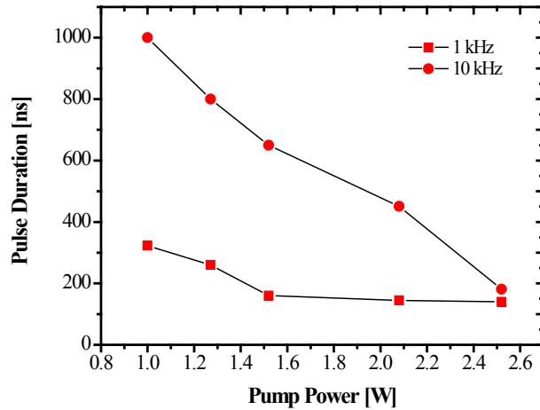
Fig. 3. Pulse duration versus launched pump power at different repetition rate.
