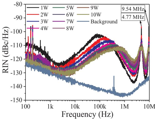
Fig. 3. RIN of the fiber laser oscillator at different power.
