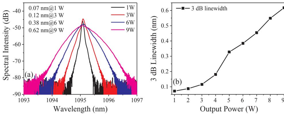
Fig. 2. Output spectra (a) and 3-dB linewidth (b) of the fiber laser oscillator at different powers.
