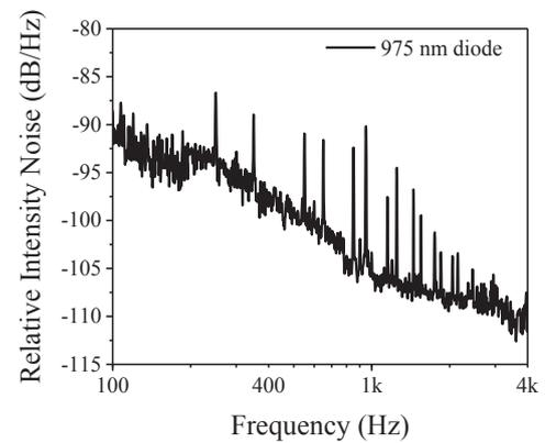
Fig. 5. RIN of a 975 nm diode laser.
