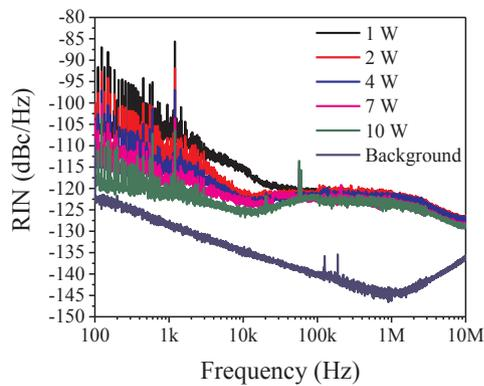
Fig. 7. RIN spectra of the ASE source at different powers.
