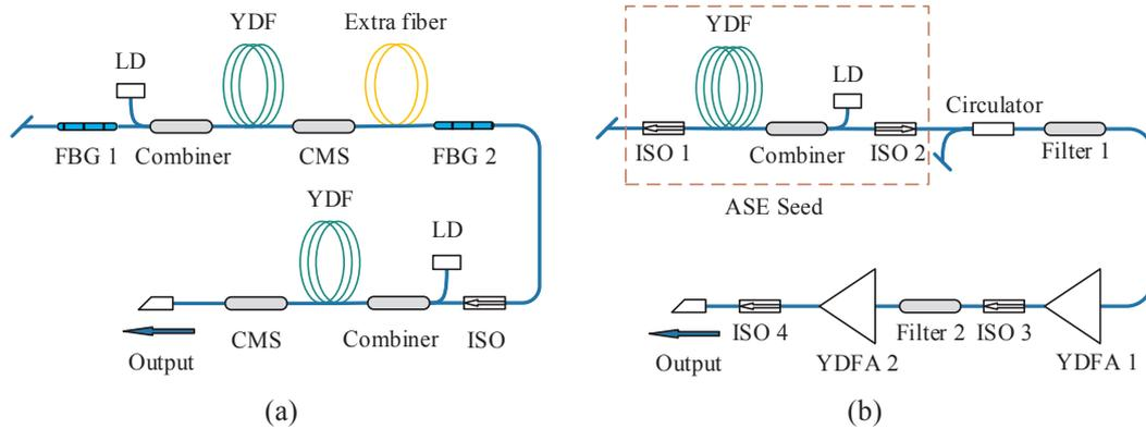
Fig. 1. Experimental configuration of the fiber laser oscillator and amplifier (a) and the fiber ASE source (b).
