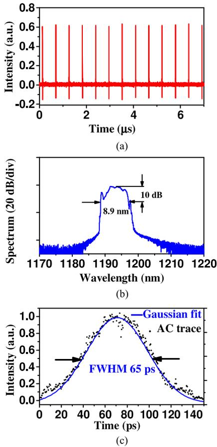
Fig. 3. (a) Pulse train, (b) output spectrum, and (c) autocorrelation trace of the mode-locked laser at a pump power of 900 mW.
