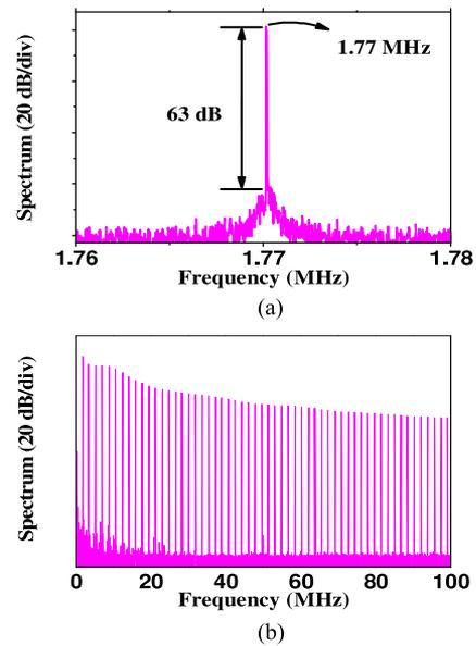
Fig. 4. RF spectrum of the mode-locked fiber laser at  $1.2 \mu\text{m}$  measured (a) around the fundamental repetition frequency and (b) in a range of 0–100 MHz.
