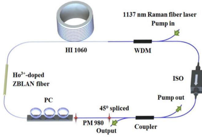
Fig. 1. Experimental configuration of the mode-locked Ho<sup>3+</sup>-doped ZBLAN fiber laser.
