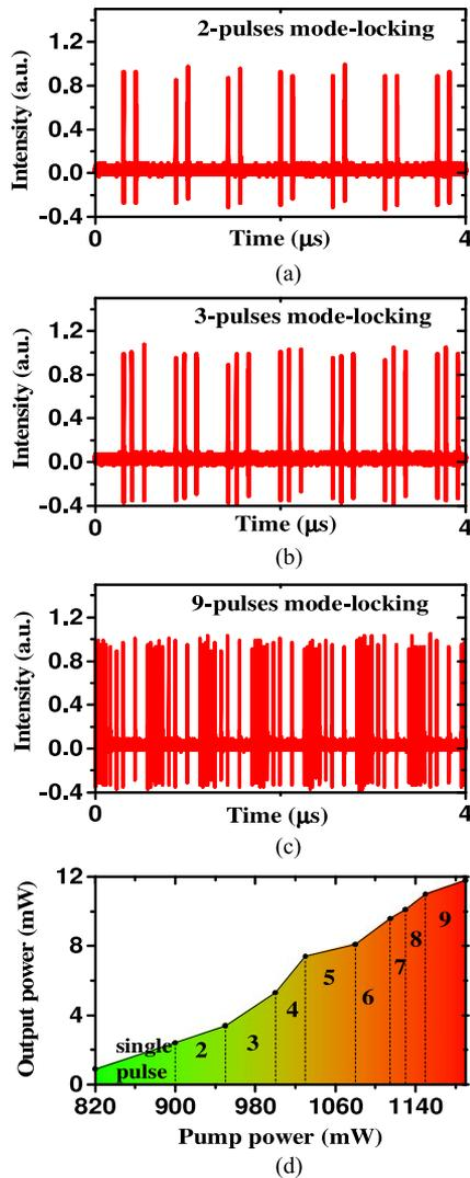
Fig. 5. Typical pulse trains of mode locking states with 2(a), 3(b), and 9(c) pulses. (d) Output power and states of the mode locking as a function of pump power.
