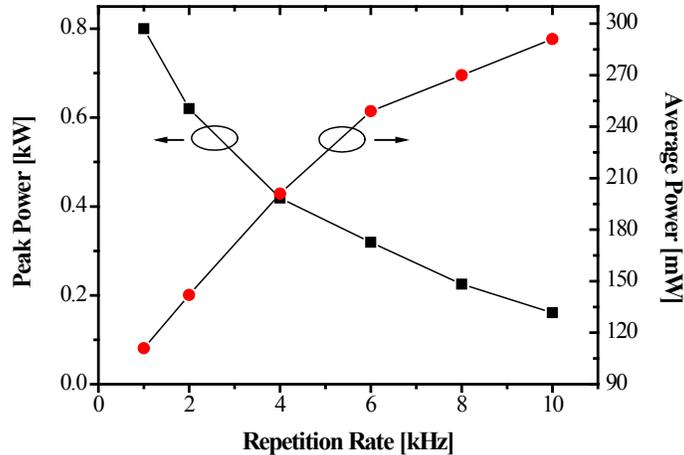
Fig. 6. The peak power and average power versus different repetition rate at pump power of 2.5 W.
