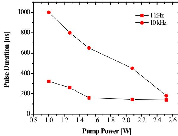
Fig. 3. Pulse duration versus launched pump power at different repetition rate.
