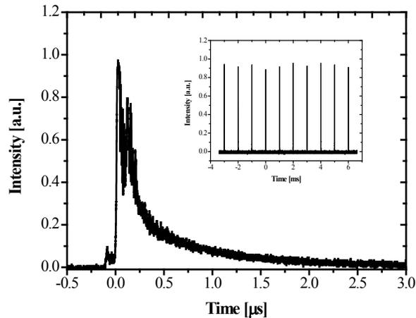
Fig. 4. Single pulse profile at repetition rate of 1 kHz. Inset, measured pulse train.
