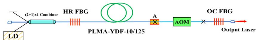
Fig. 1. Experimental configuration of Q-switched fiber laser at 1120 nm.
